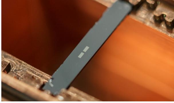
Figure 3.6: **Picture of a transmon inside a 3D cavity.** The large shunting capacitors (light gray) are clearly visible on the silicon substrate (dark gray), whereas the Josephson junction in between them is too small to be seen. The substrate is mounted in a copper cavity.
