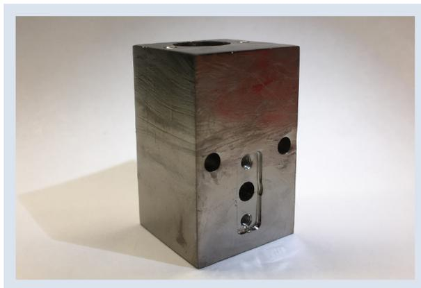
**Figure 4.8:** Picture of the high purity niobium coaxial quarterwave resonator, after the BCP surface treatment.
