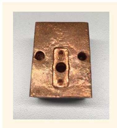
**Figure 4.4:** 6N copper cavity after 1h FeCl etch treatment. The impact of the inhomogeneous etching treatment can be seen in the rough and distorted surface.
