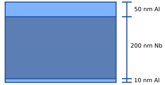
Figure 4.11: Triple-layer structure of the ground plane.
